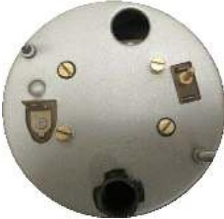
This is the Gen-1 OEM tachometer which has one of the power supply connections electrically connected to the metal case. In many cases the "red-line" will be marked on the dial but not always. Similarly, polarity will be generally be marked on the dial as shown but this also may not always be the case.
