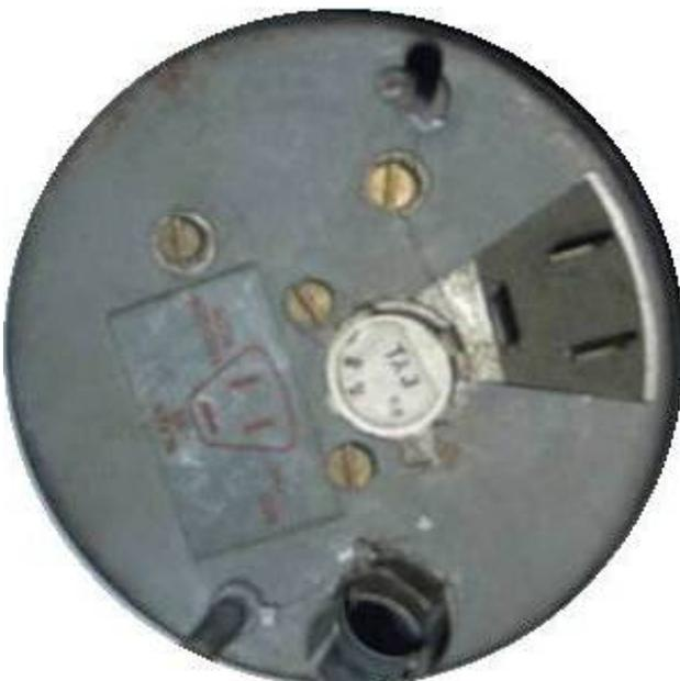
Note the white selector switch next to the terminals. This selector switch is only found on Gen-4 instruments, Gen-3 RVC tachometers used a switch accessed through a hole in the rear of the case.
